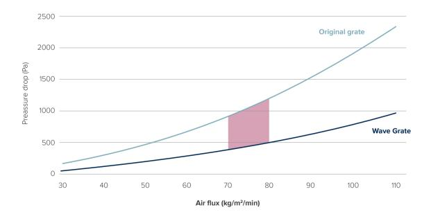
Based on industrial tests on a SF Cross-Bar cooler, the typical operating air flux range of 70–80 kg/m²/min, the pressure drop across the grates is reduced by ~60%, and the total pressure drop of the fan is reduced by ~8%.
